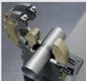
/ Perfect welds due to closed chamber
