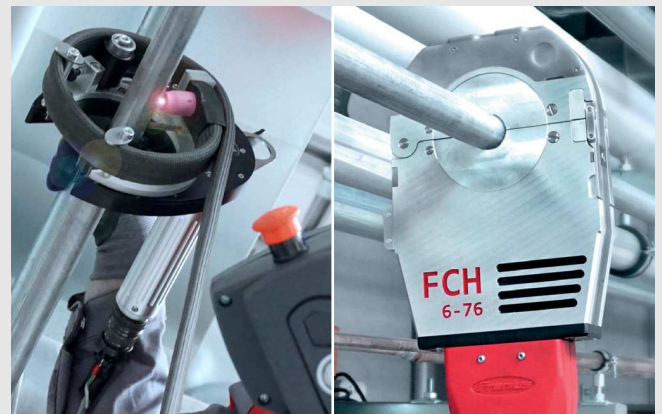
/ open and closed weld heads FOH / FCH in use
