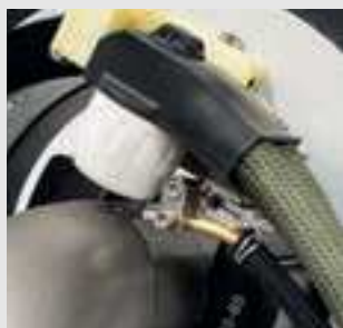
/ Wire feeding, torch bracket from 0 - 45° stepless swivelling
