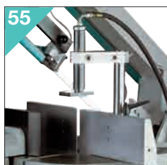
55 XT40002 BS 350 - 400 SHI Morsa idraulica verticale lato scarico. Hydraulic vertical vice, unloading side.
