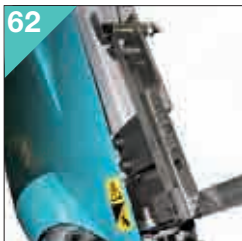
62 Controllo deviazione lama. Device to check the blade squareness/accuracy.
