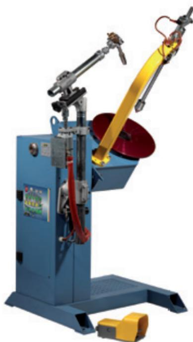
with pneumatic tailstock for the locking of the piece to be welded and with manual tilting through wheel with reduction unit.
