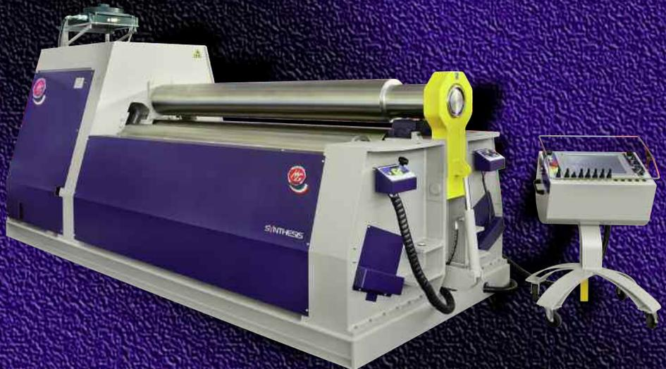
3-roll plate bending machines, for sheet thickness from 1 mm up to 300 mm, very easy to operate. **G** with planetary side roll system and parallelism controlled by torsion bars, **GE** with electronic parallelism, **GL** Electronic parallelism and side rolls moving on linear guides.
